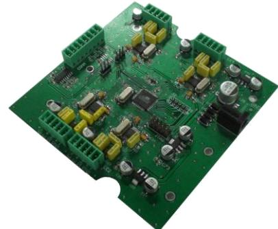
Each load cell channel is supported by an independent 24 bit  $\Sigma\Delta$ - Analog-to-Digital Converter, special linearity compensation method plus all other state-of-the-art technologies applied, all these together enable **DJB** to provide fast, stable and almost error-free weighing result at anytime and anywhere.
